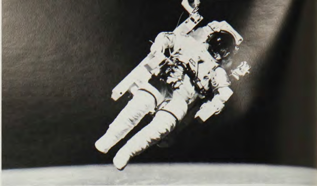
► The manned maneuvering unit allowed space walks during the 1984 Shuttle Challenger mission. Astronaut Bruce McCandless was the first to use the apparatus.
